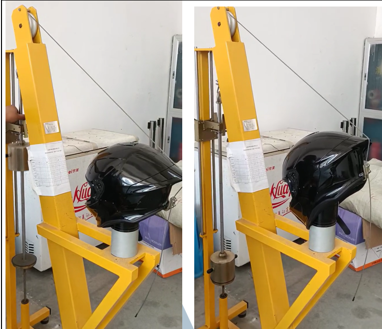
Retention detaching test
